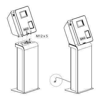
Screw the bottom plate into the interior structure
