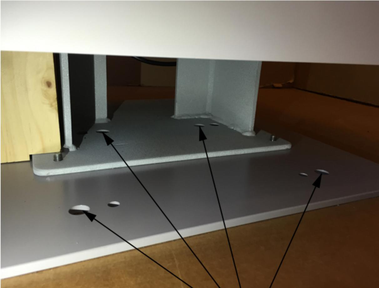
Fix the machine to the floor with provided M12 bolts and anchors.
