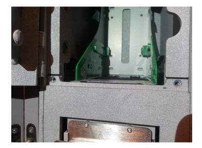
5. These screws hold in a metal plate. Tilt the top of the plate towards you, and pull it upwards and outwards. Note: you may need to push on the bill validator mouth as there are two white plastic parts which can block the metal plate from being removed.
